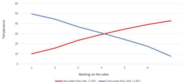
**Three-way valve temperature setting**
